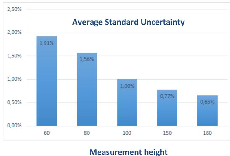
*Standard uncertainty of all AQ510 in analysis with EPs according to IEC. AQ510 has been classified according to the procedure described in Annex L of the IEC guidelines, 61400-12-1, and achieved a mean standard uncertainty of 1,00% at 100m.*
